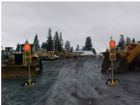
RDTL System with four 12" head units, microwave vehicle detector. Operating a 1,200 feet zone
