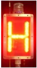
Dual Direction, Single Digit Display used for informing personnel of conditions before entering an area
